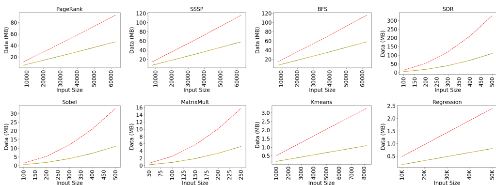
Fig. 18. Effect of input size on communication volume. Dashed red line is the baseline, orange line is Diamond.
